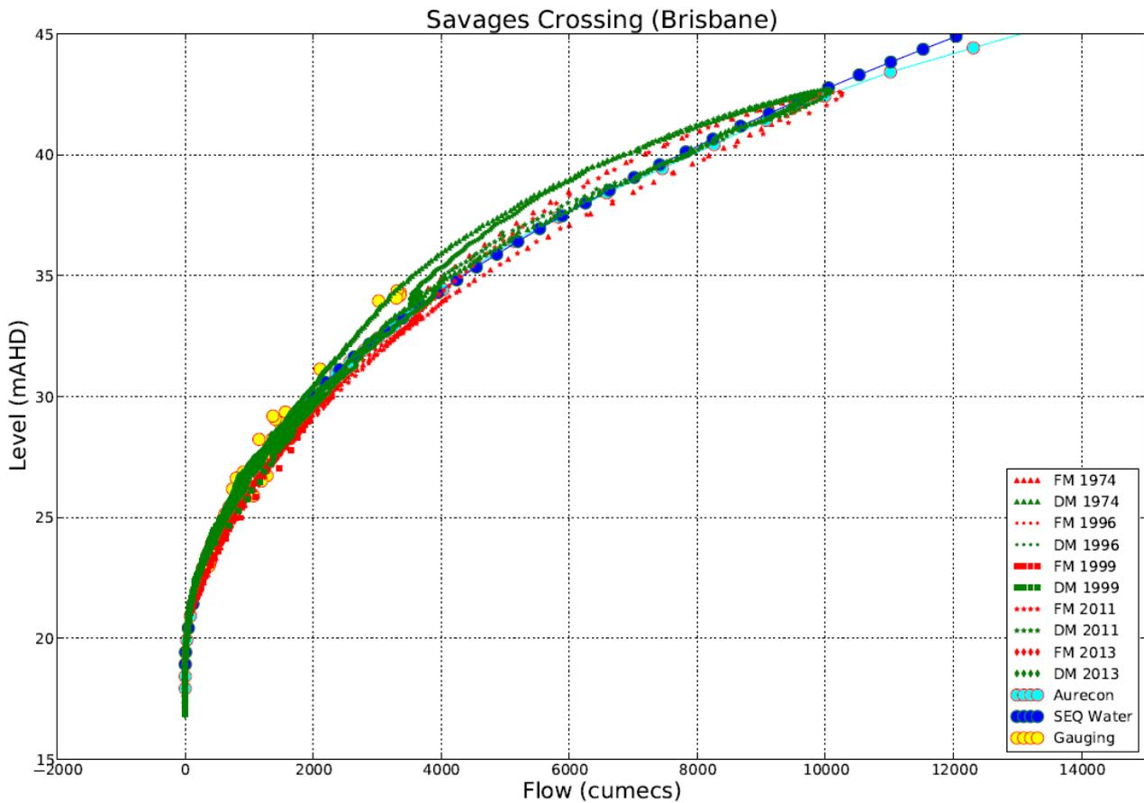
Figure 6-8 Rating Curves versus Hydraulic Modelling Calibration Results – Savages Crossing
