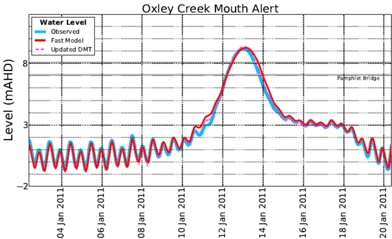
Figure 5-2 Example of Plot Output showing both Updated DMT and FM results
