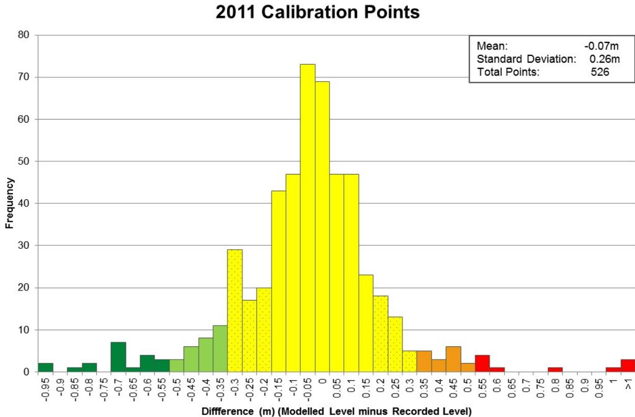
**Figure 6-6 2011 Detailed Model Calibration - Statistical Assessment of Differences between Observed & Modelled Peak Flood Levels**
