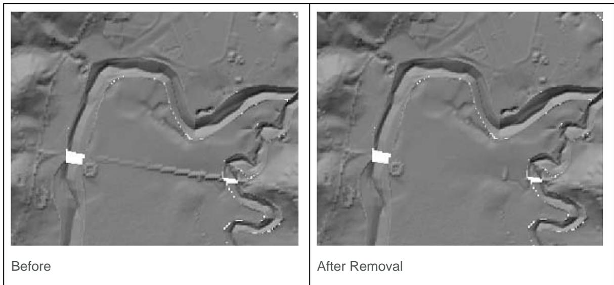
Figure 6-1 Removal of Cunningham Highway Raised Section for 1974 Topography
