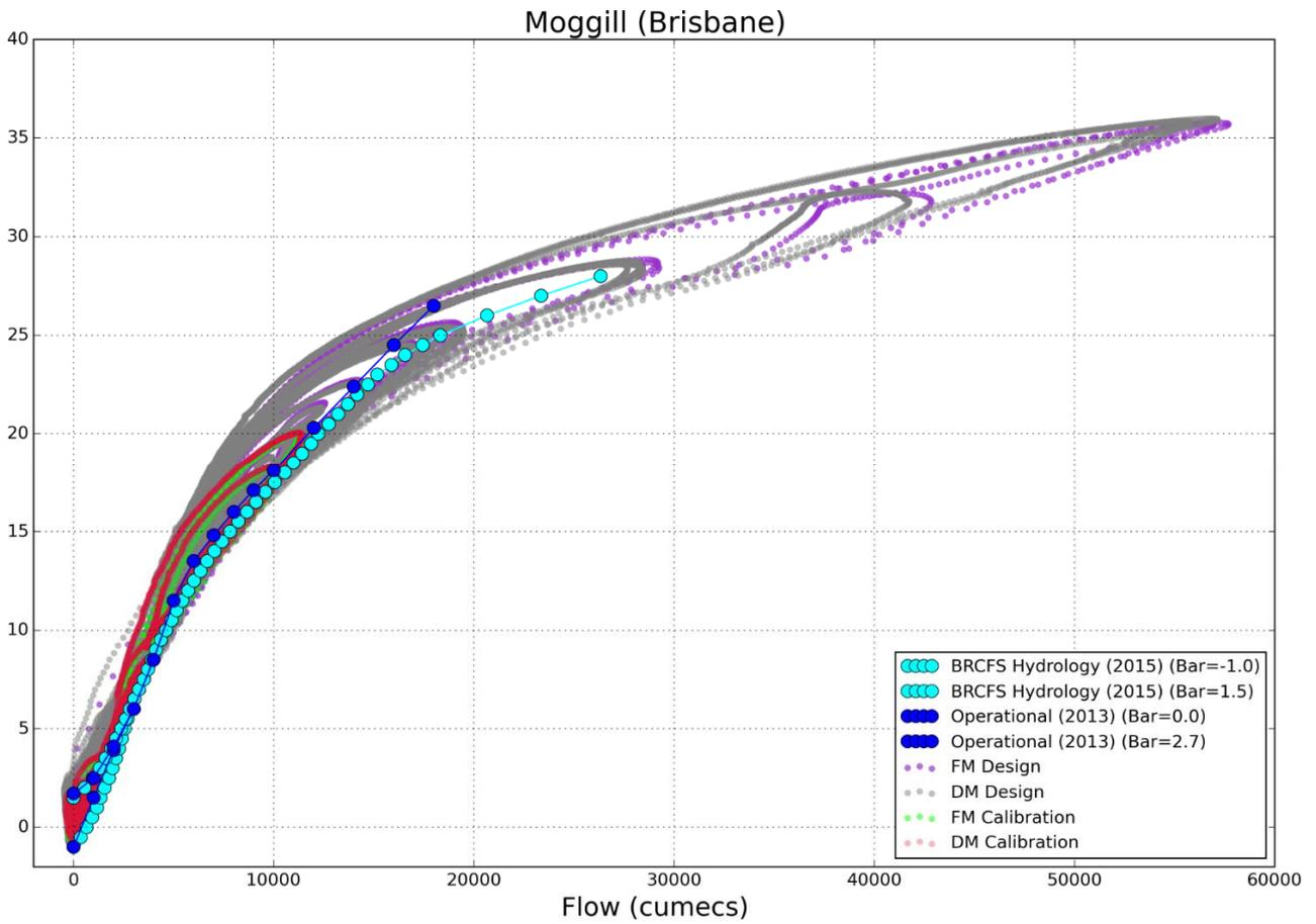
Figure 8-11 Rating Curves versus Hydraulic Modelling Calibration Results – Moggill
