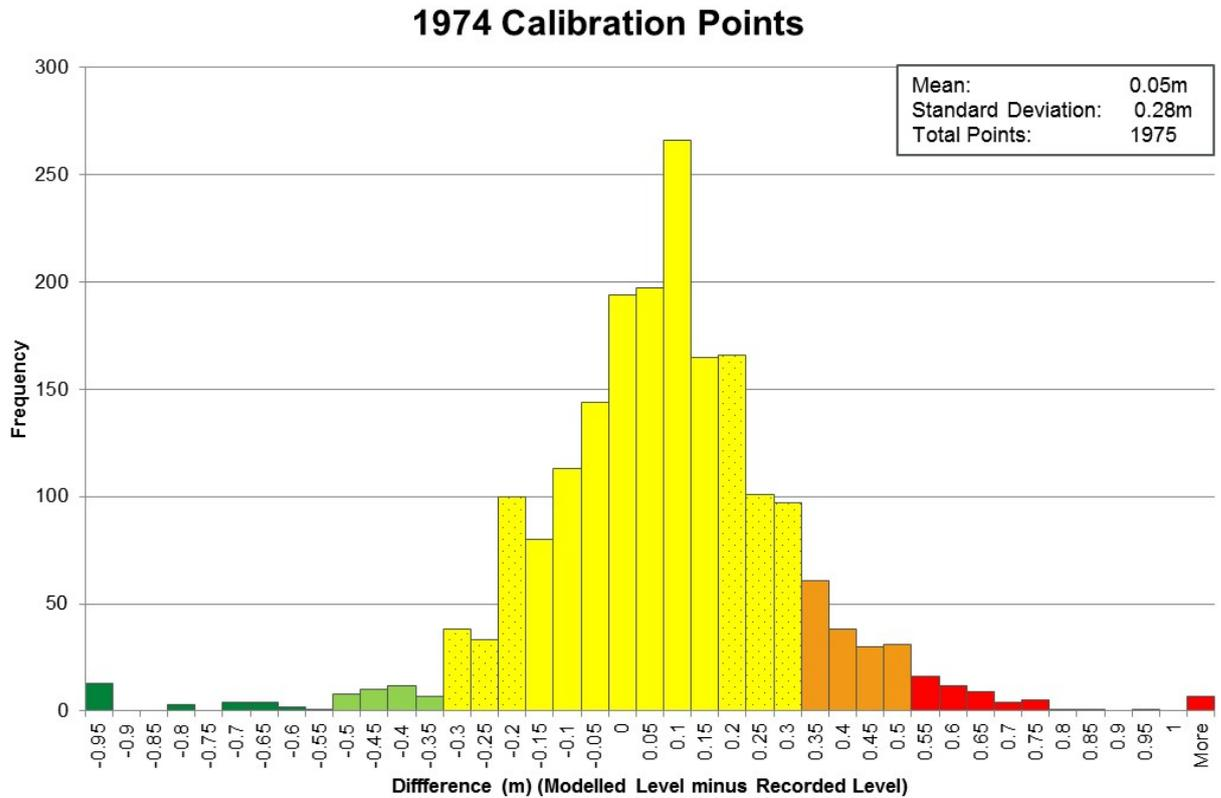
Figure 6-7 1974 Detailed Model Verification - Statistical Assessment of Differences between Observed & Modelled Peak Flood Levels
