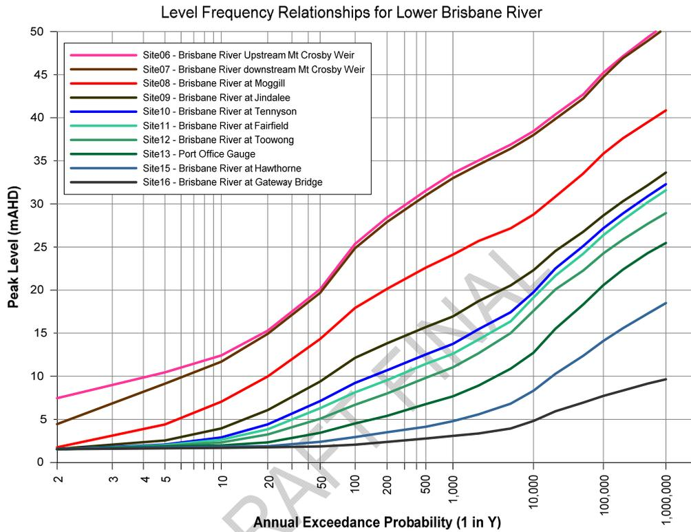
Figure 7-4 Derived Level Frequency Relationships for Sites along the Lower Reaches of the Brisbane River
