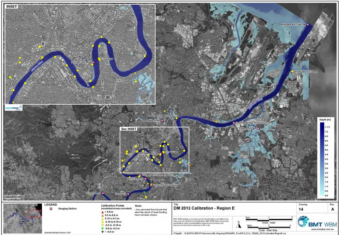
Figure 3-4 Example Map Showing Calibration Points (Flood Marks)
