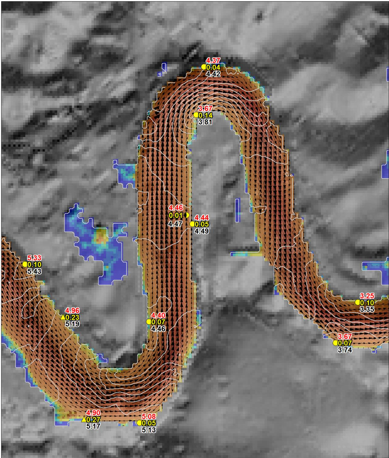
Figure 6-5 Example of Reproduction of Superelevation at River Bends for the 2011 flood – Story Bridge Bend
