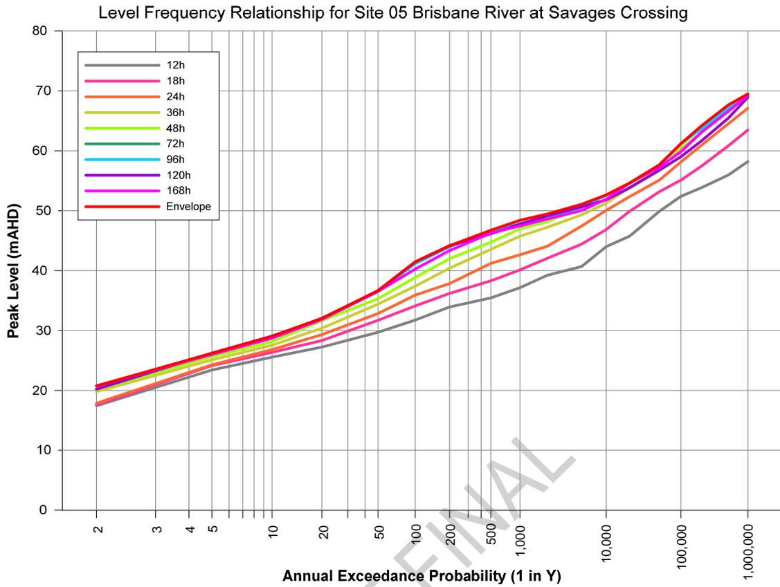
Figure 7-3 Example Frequency Relationships for All Durations at Savages Crossing, and the Envelope of Level Maxima with AEP
