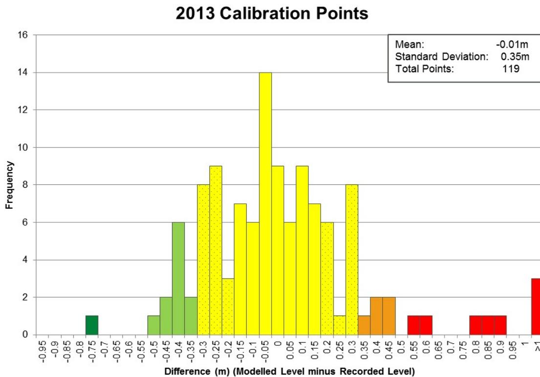
**Figure 6-4 2013 Detailed Model Calibration - Statistical Assessment of Differences between Observed & Modelled Peak Flood Levels**
