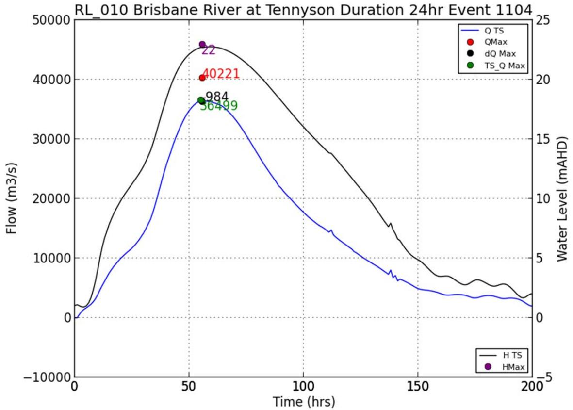
Figure 7-1 Example Plot Used to Identify Numerical Instabilities
